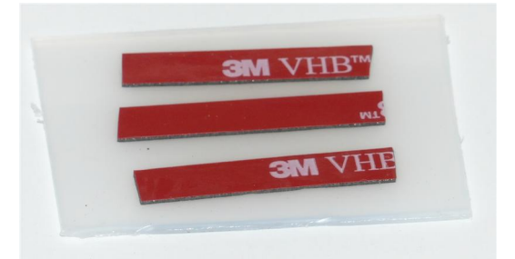
3M VHB tape to secure pot cable
