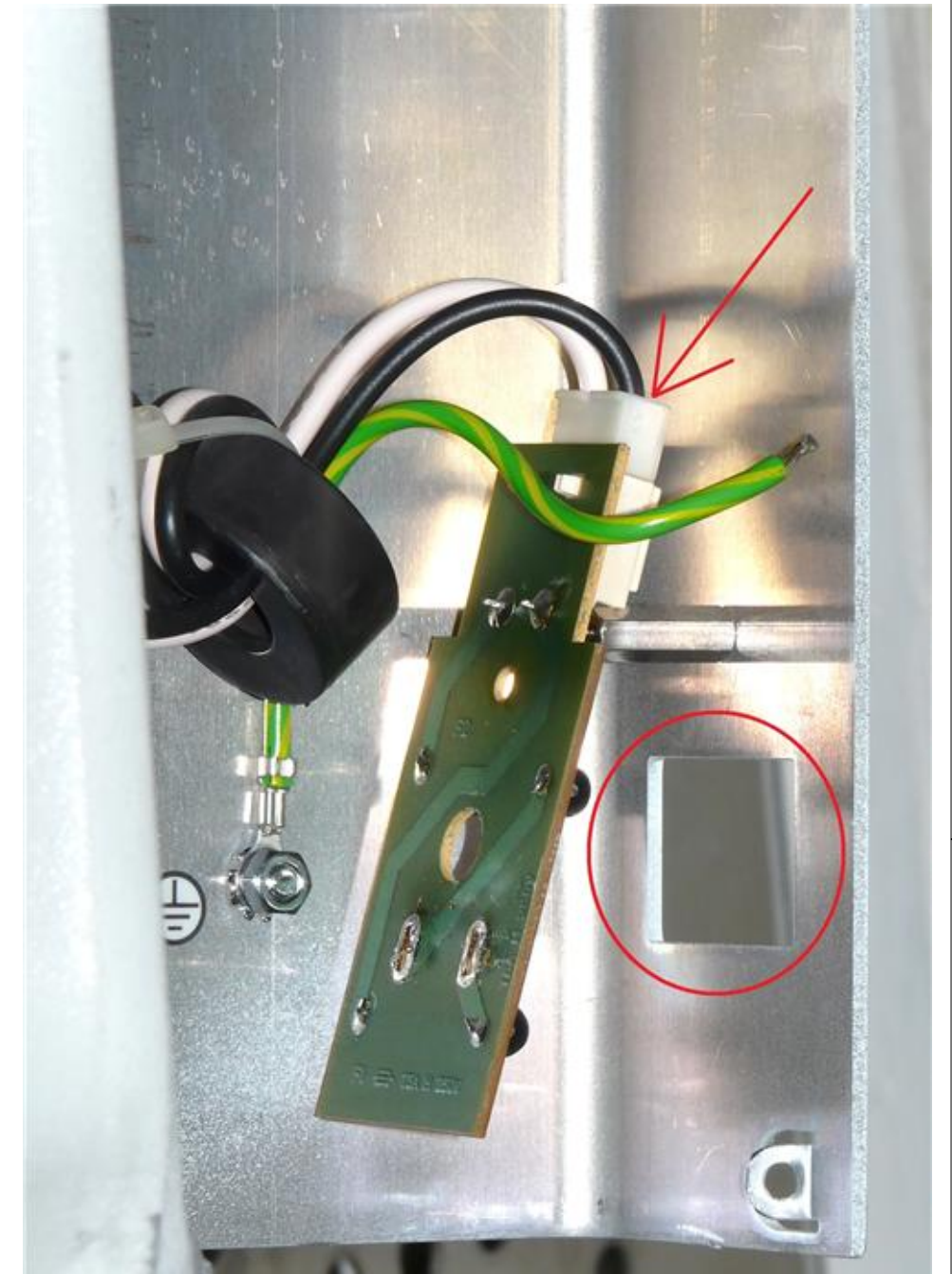
(1) Inside view of obsolete AC power input for BX51-61. (The AC input receptacle which would be mounted in the empty circled hole had been removed before we received the microscope) Remove AC power lead connection by disconnecting the socket indicated by the arrow above.
