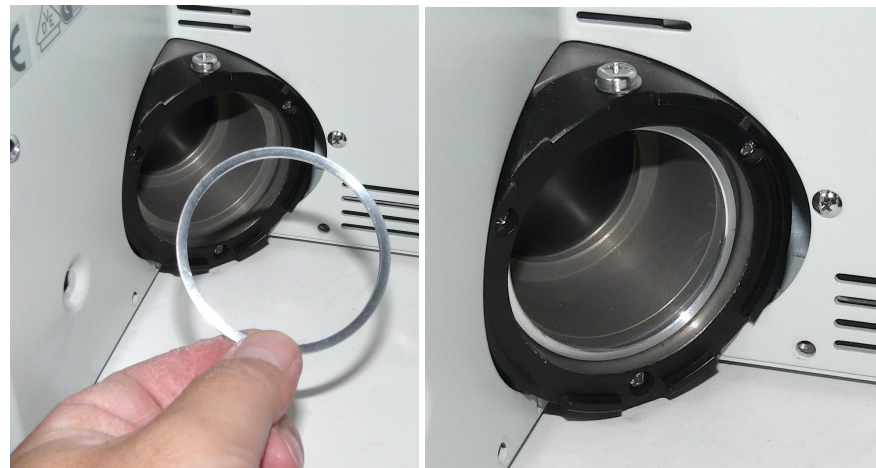
(2) Place the spacer in the port. To keep it in place, either tilt the microscope or the spacer so it doesn't fall out. The spacer shown here is aluminum but yours may be a different material. (photos are a BX50)
