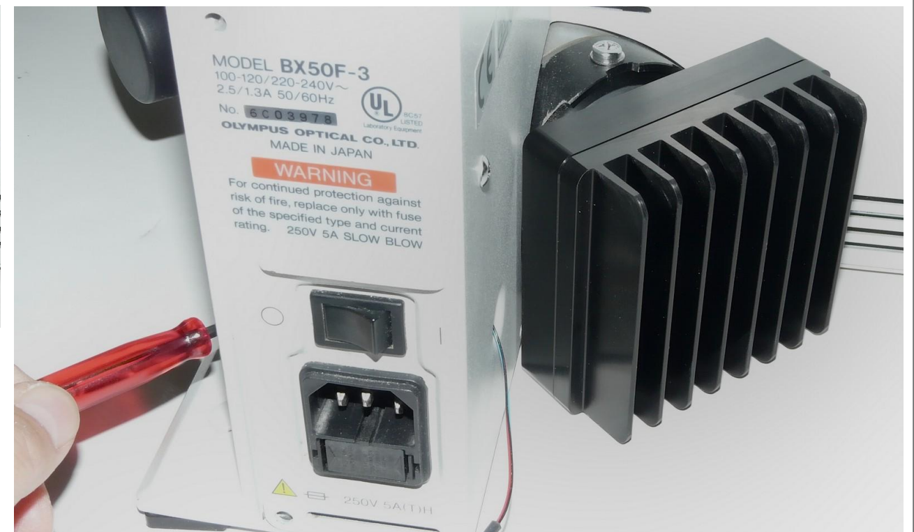
(3) Insert the illuminator into the microscope port and secure it the same way as the original. Keep it pressed firmly in place until the microscope screw has secured it, to ensure good alignment. (The photo is a BX50. For the BX51-61 the pot cable should be coming out under the illuminator.)
