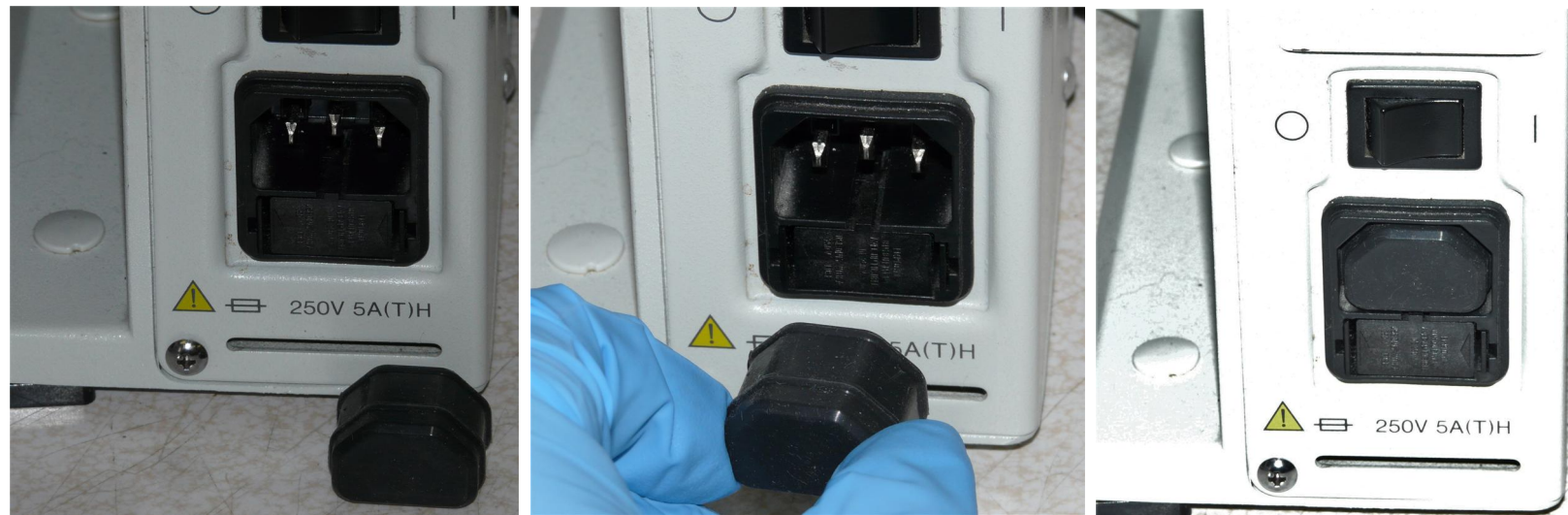
(2) Installing PN 10736 rubber plug in AC receptacle to deter connection of obsolete AC power.
